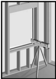
Squaring (window frame)
